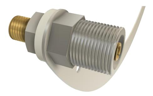
3) Next place the stainless washer on the stud, next to the hex nut, followed by the other element with the smaller hole. Using the remaining hex nut, complete the feeder point assembly, keep this nut loose for now. The connector and elements should look like the following photo, less the black plastic fasteners and spacers.
